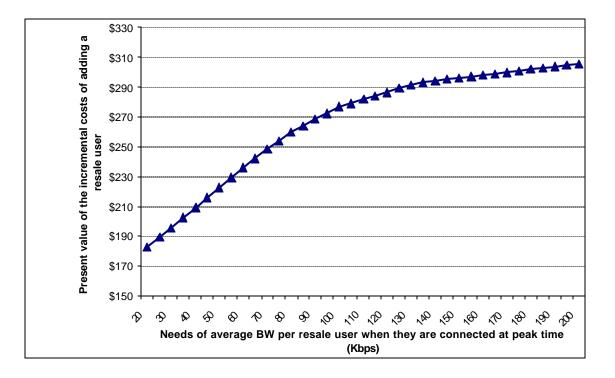
Figure 13: Sensitivity of the PV of incremental costs to the needs for peak average bandwidth of the resale users (expanded variation range)
