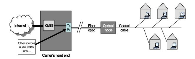
Figure 2: Simplified architecture of an HFC network
