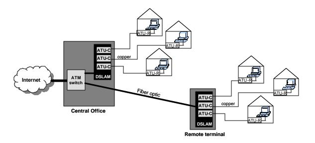
Figure 1: Architecture for the ADSL-based access network<sup>36</sup>
