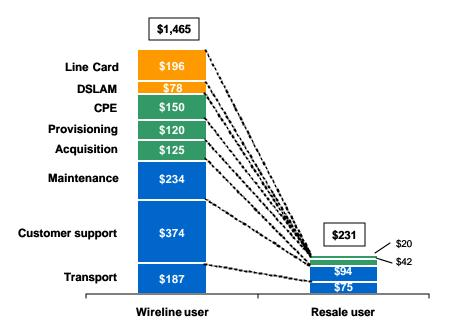
Figure 11: Present value of incremental costs to the carrier for addition of a wireline user and a resale user<sup>208</sup>
