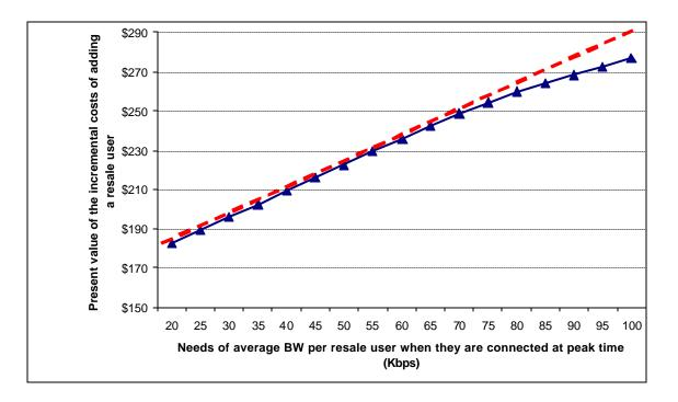
Figure 12: Sensitivity of the PV of incremental costs to the needs for peak average bandwidth of the resale users
